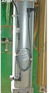
Balluff's V-Twin magnetic field sensors provide two sensors with a single connector. Realize substantial savings on installation cost with only one four conductor cable, less installation hardware, and fewer terminations. The new BMF V-Twin is available in several sizes and form factors to cover applications from grippers and short stroke cylinders to C-Slot, T-Slot, round, and tie rod cylinders—in some cases without requiring additional mounting brackets.
