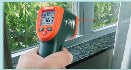
Checking for heat loss around windows and doors
